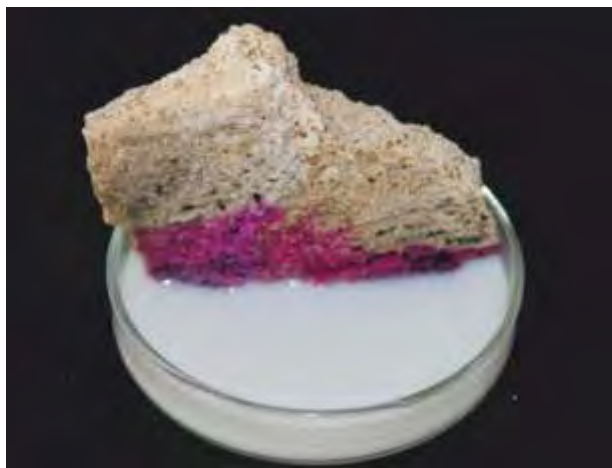
Figure 5: Phenolphthalein indicating the diffusion of CaLoSiL® E25 into a porous mortar sample.
