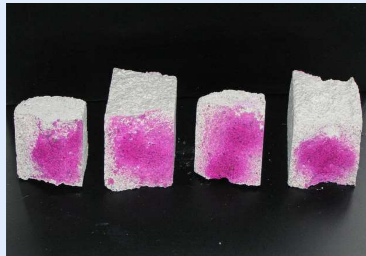
Alkaline reaction of mortar samples after the treatment with Nano-lime
