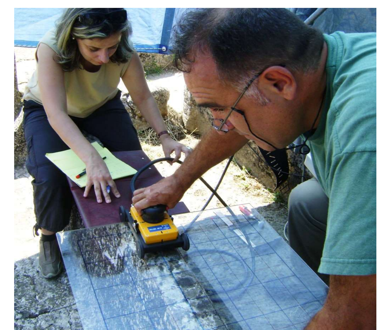
Non-destructive stone assessment by using Georadar
