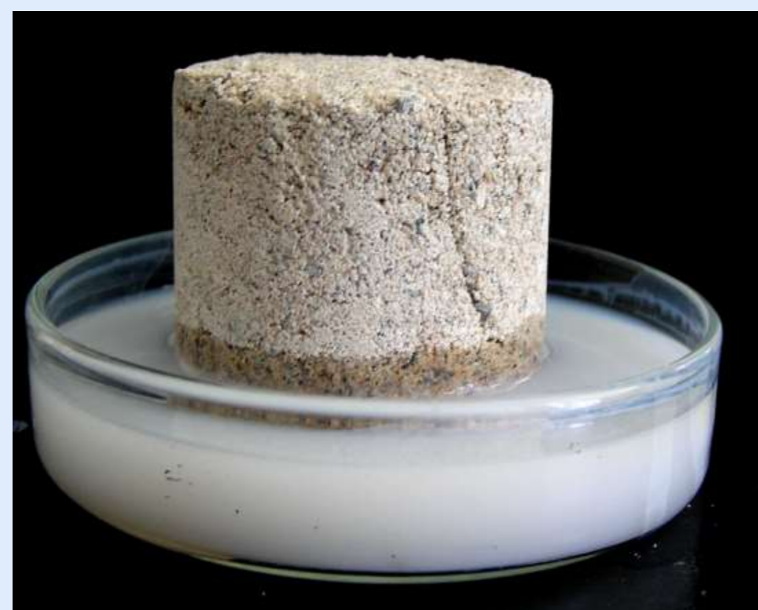
Alkaline reaction of mortar samples after the treatment with Nano-lime
