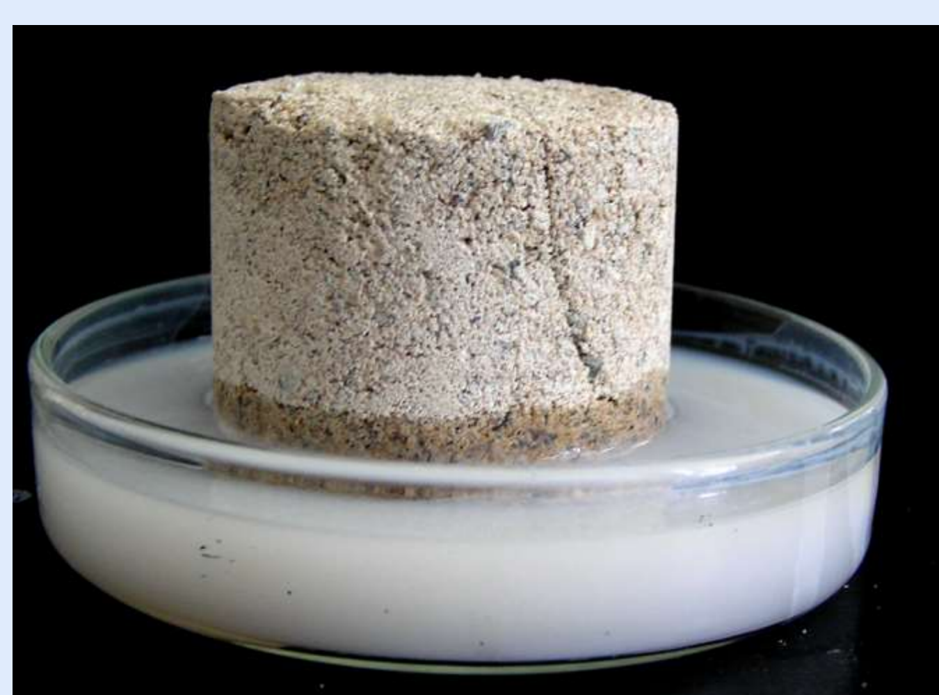
Penetration into mortar
